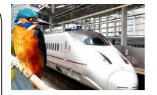
Using a Kingfisher's head and bill profile as inspiration, the redesigned Japanese bullet train created less drag and friction when travelling and didn't create a sonic boom on exiting tunnels.
