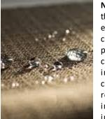
Nanomaterials are exceptionally thin materials. The are used in electronics to improve conductivity and allow the production small of verv components. In the textiles industry they can add protective coatings to improve water resistance, UV protection and improve anti-bacterial protection in footwear.
